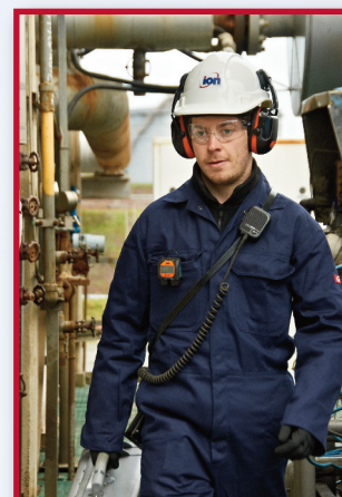
Cub TAC personal PID monitor worn to provide continuous detection.
