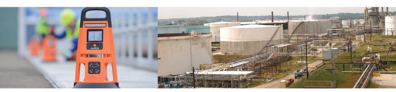
Tanks farms are used to hold a wide range of products. In the headspace of each of the tanks within the farm, any number of toxic or combustible gases may be present. Radius BZ1 Area Monitors can be set up near a tank farm to make sure those toxic or combustible gases are not escaping into the environment.
