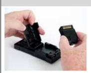
Step 5 (ER). Unlatch and lift the cradle lid; remove the battery. Close the cradle lid; set aside the charger adaptor for future use.
