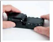
Step 2. Press down on the battery pack to secure the battery to the charging surface; a click will sound.
