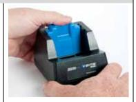
Step 3 (ER). Place the charger's insert into the charger's back slot.
