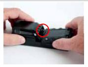
Step 1. Place the battery pack onto the charging surface at the angle shown (approximately 30 degrees).
