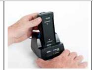
Step 5. Lift the battery bottom at the angle shown (approximately 30 degrees); remove the battery from the adaptor. Set aside the charger adaptor for future use.
