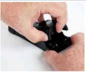
Step 1 (ER). If a battery pack is attached to the adaptor, remove it (see step 5 above). Press the cradle latch. Lift to open the extended range battery cradle.
