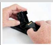
**Step 2 (ER).** Place the battery into the **charging cradle**, circuitry side facing down.
