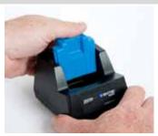
**Step 3**. Place the charger's insert into the charger's **front slot**.
