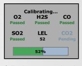
Calibration progress and results are shown for each sensor.
